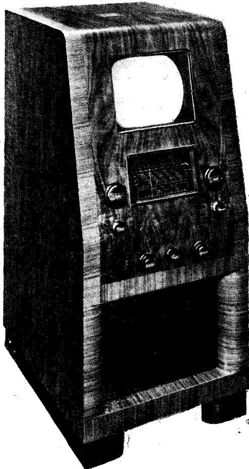
The H.M.V. Model 907 vision and all-wave sound equipment with a 9-in. tube.
