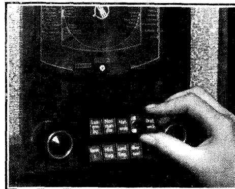
Philips push-button system: removable cover on button gives access to pre-set tuning adjustment.
